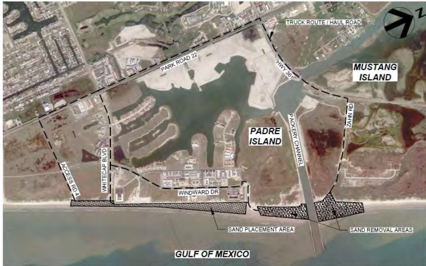
Figure 7. Temporary Truck Routes/Haul Roads for Sand Relocation.
