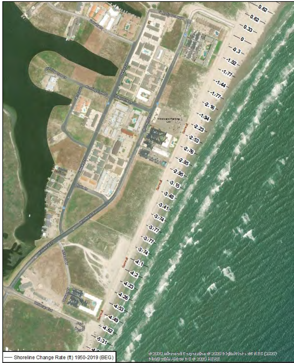
Figure 3. Historical Shoreline Change Rate (feet/year) at the NPI Seawall (data provided from BEG [Paine and Caudle, 2020]).
